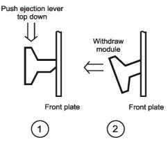
Figure 2: Function of the ejection lever
